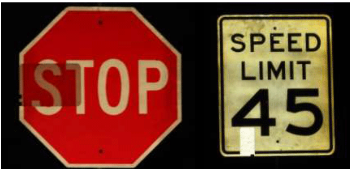
Figure 1: Examples of comparison panels on traffic signs that pass (left) and fail (right) (1)
