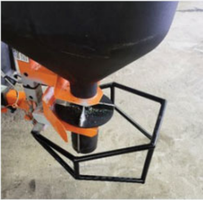
Swatara Township Highway Department, Pennsylvania Steel Guard Keeps Salt Spreader Out of Harm's Way
