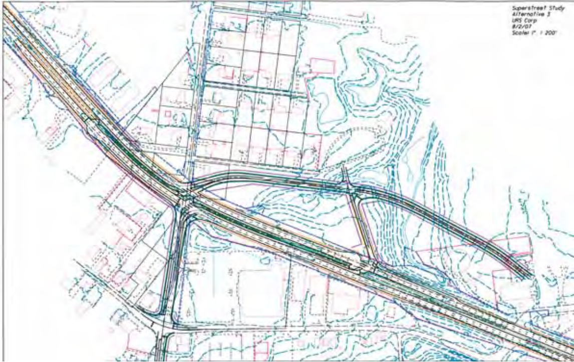
Figure 224. Illustration. Proposed configuration at the intersection of U.S. Route 32/Bells Lane intersection used in case study.
