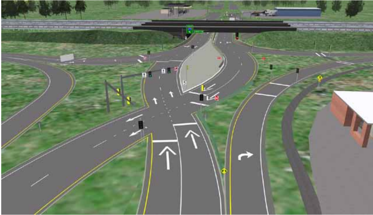
Figure 160. Illustration. Crossover of a simulated DCD interchange.
