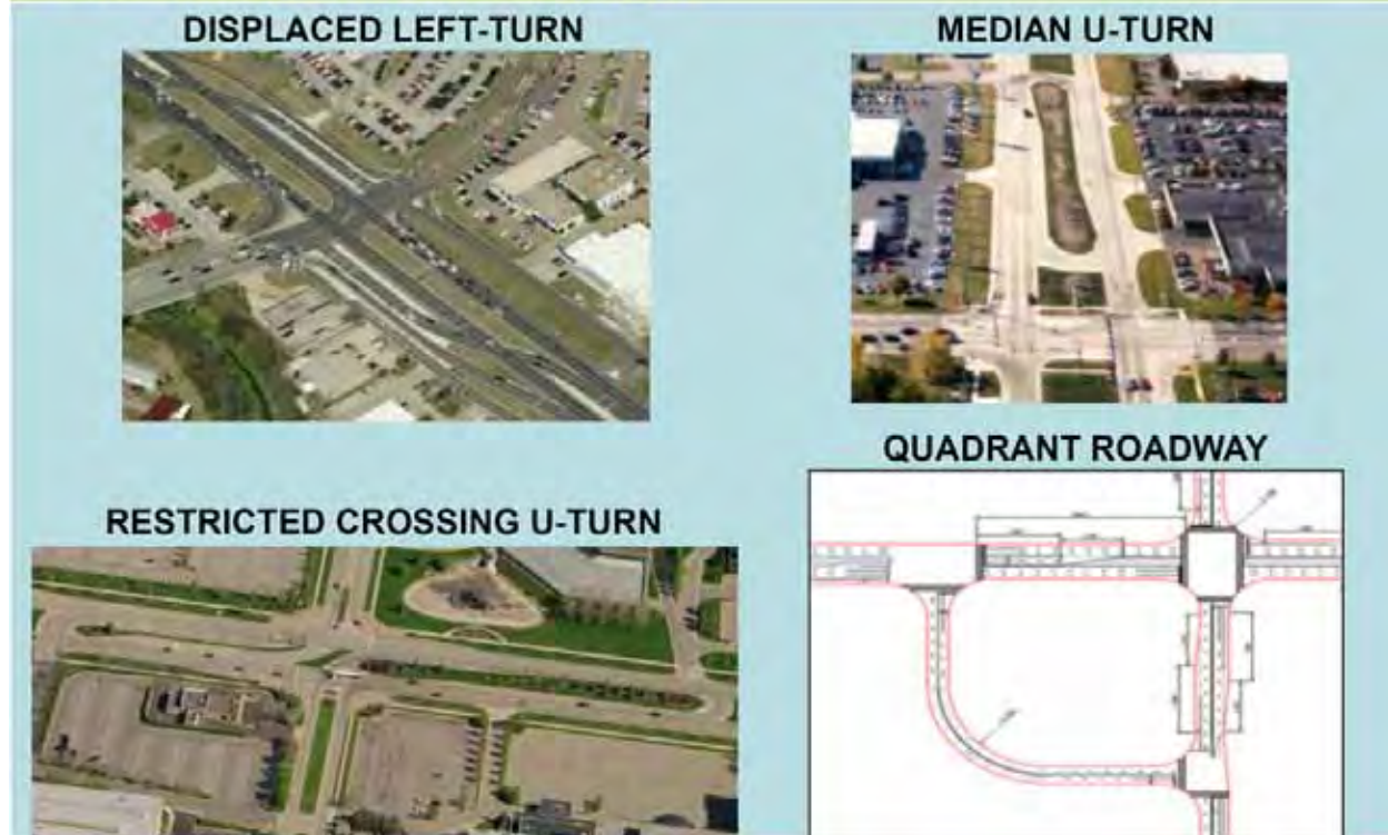
Figure 1. Photo. Four alternative intersection configurations.
