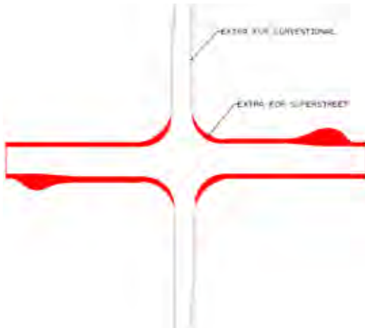
c. Footprint comparison of a RCUT versus a conventional intersection with narrow median and two through lanes for side street.
