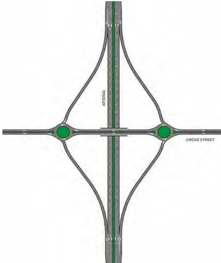
Figure 199. Illustration. Double roundabout interchange. (4)
