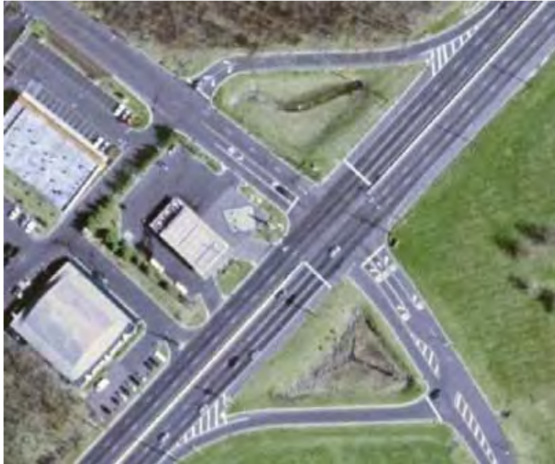
Figure 144. Photo. Typical jughandle intersection in New Jersey.
