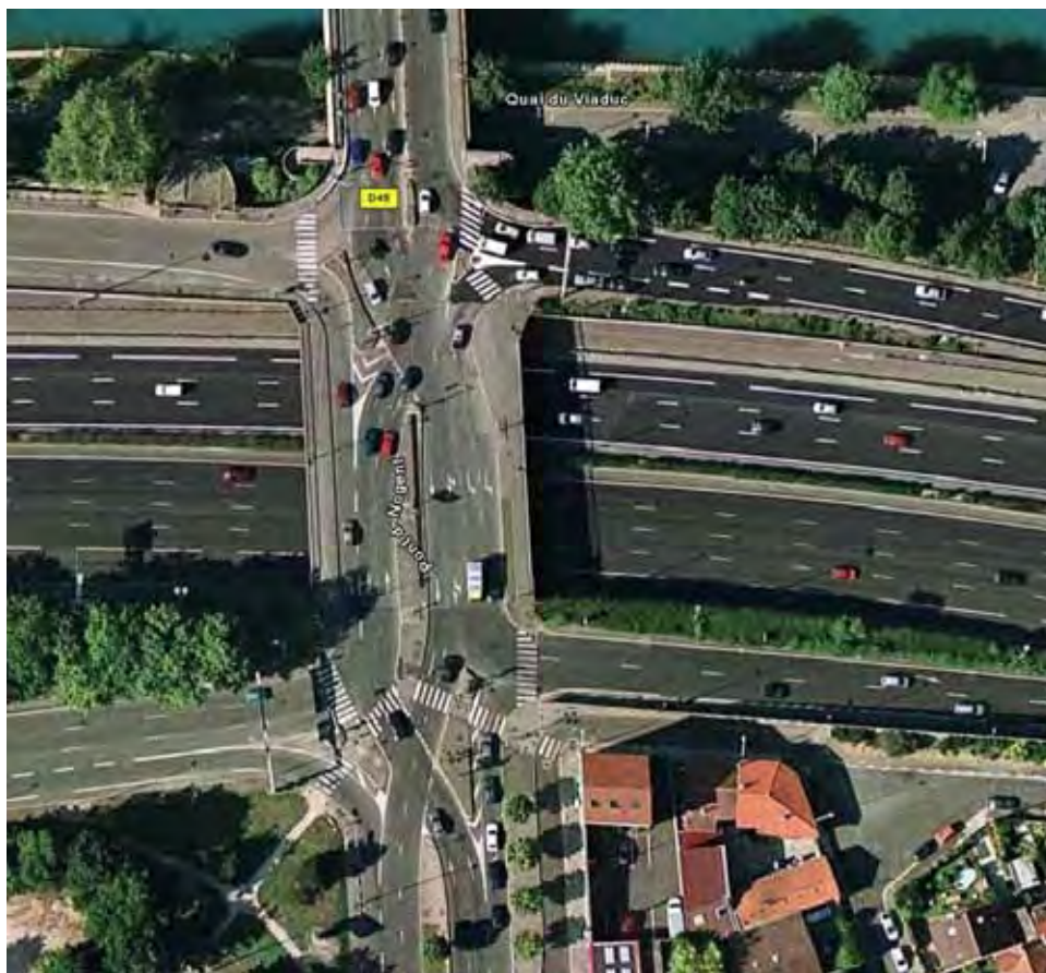
Figure 157. Photo. DCD interchange in Perreux-sur-Marne, France.
