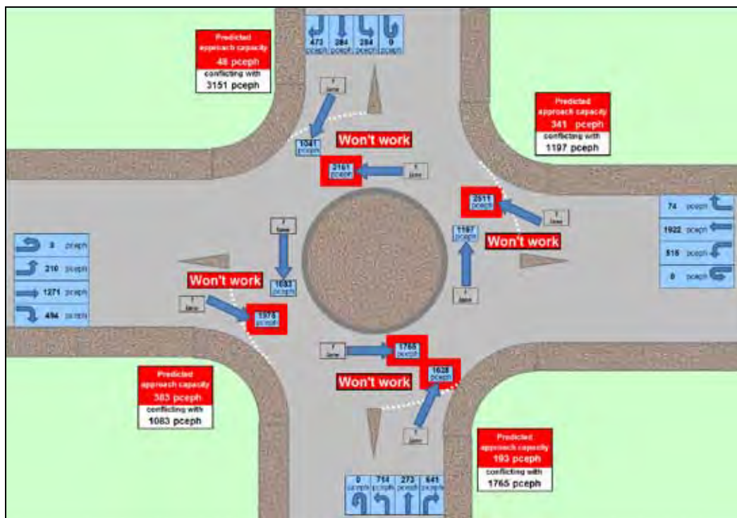
Figure 214. Illustration. Spreadsheet tab pertaining to a one-lane roundabout.
