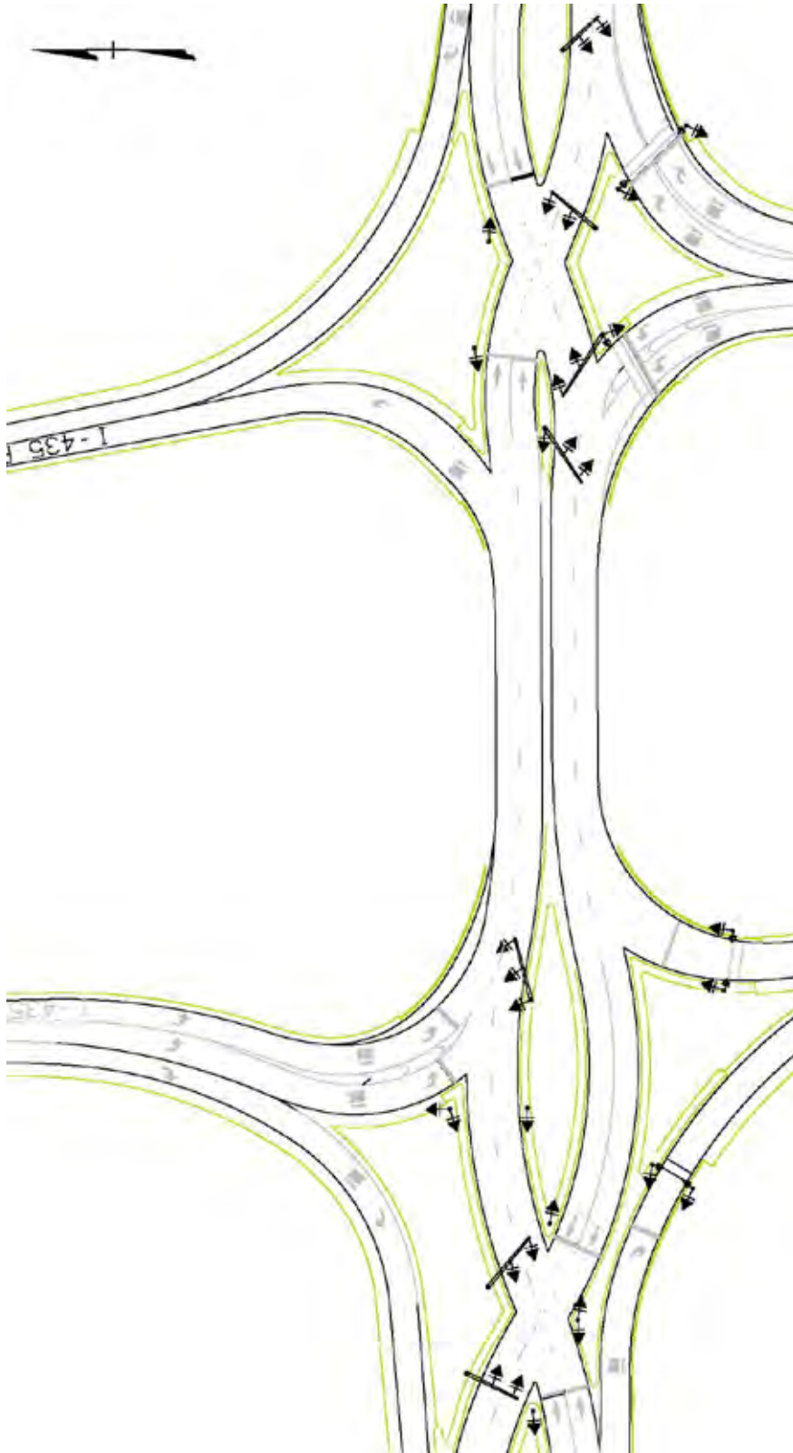
Figure 167. Illustration. Signal mast arm and pole locations being implemented in Kansas City, MO.
