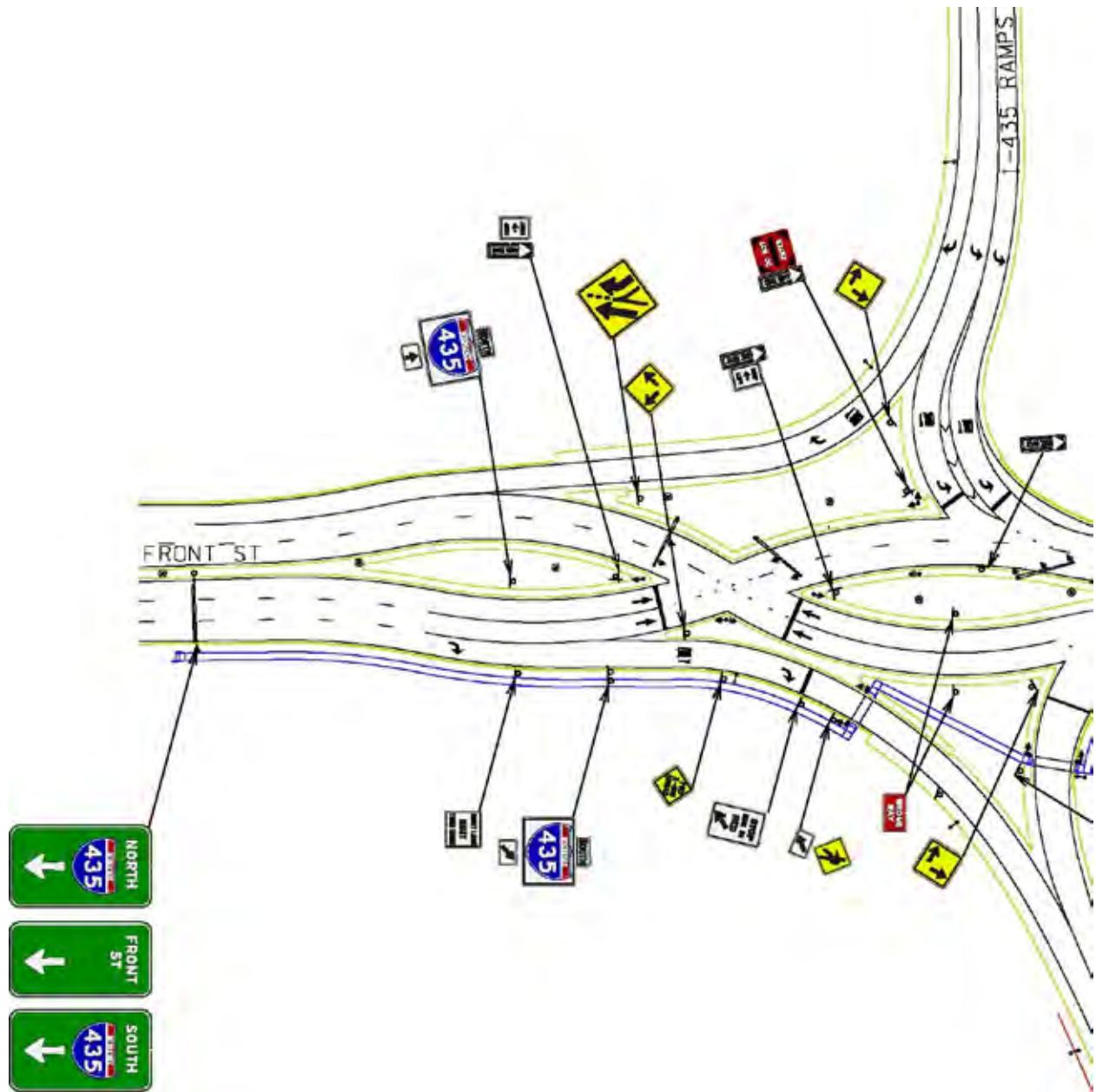
Figure 172. Illustration. DCD interchange signing and marking plan derived from Missouri practice—west end.
