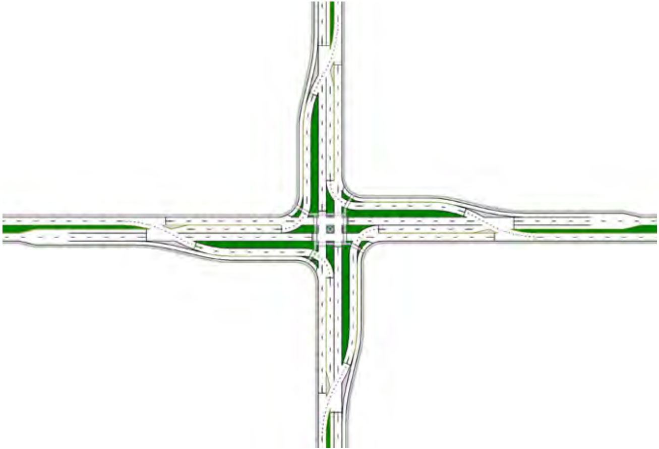
Figure 151. Illustration. Typical geometry of a parallel flow intersection.
