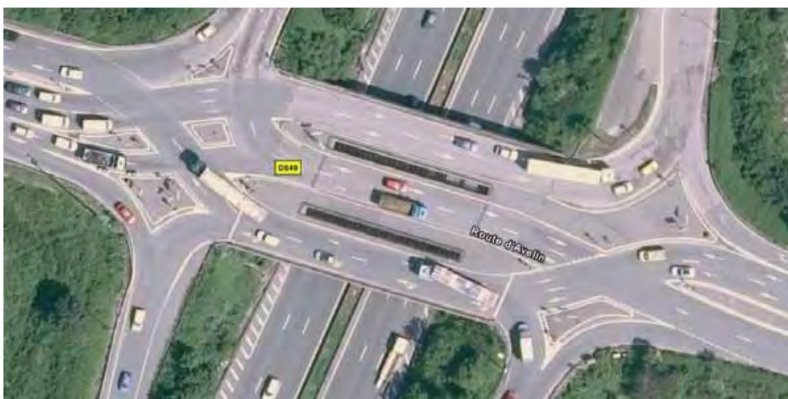
Figure 158. Photo. DCD interchange in Seclin, France.
