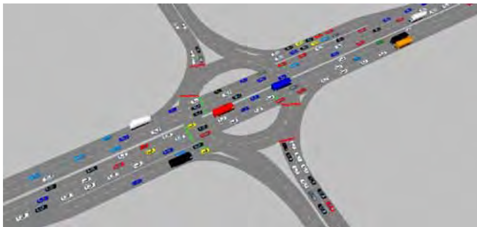
Figure 145. Photo. Typical hamburger intersection movements. (75)
