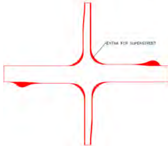
b. Footprint comparison of a RCUT versus conventional intersection with wide median and single through side street.
