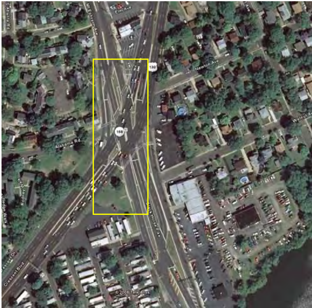
Figure 152. Photo. Aerial view of parallel flow intersection in Oaklyn, NJ.
