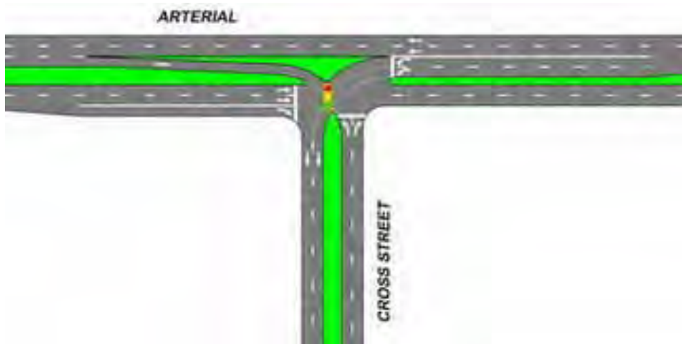
Figure 149. Illustration. Typical geometry of a continuous green T-intersection. (4)
