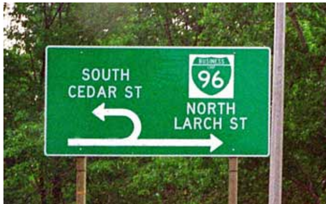
Figure 70. Photo. Example of minor road signing used at an MUT intersection in Michigan.
