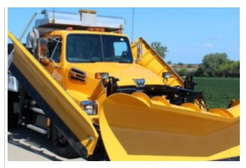
hydraulic system and spreader, 360-degree LED emergency lighting, LED wing lights, and rubber cutting plow edges with a blade saver on the front plow.
