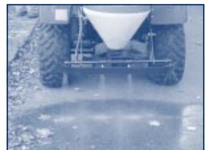
A steady stream of a de-icing agent can be applied to sidewalks or roadways.
