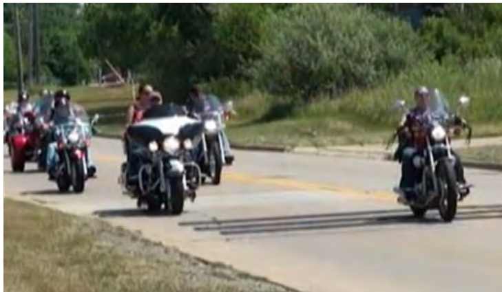
Figure 2. Motorcycles crossing Portable Reusable Rumble Strips at the BALD charity motorcycle run.
