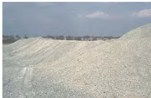
Figure 30. Photo. Aggregate for asphalt concrete.
