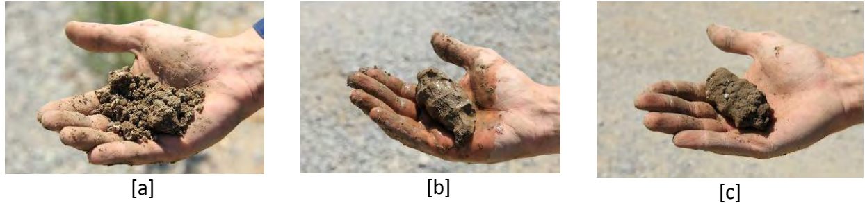
Figure 64. Photo. Squeeze test for assessing moisture content. ([a] too dry, [b] too wet, and [c] acceptable)
