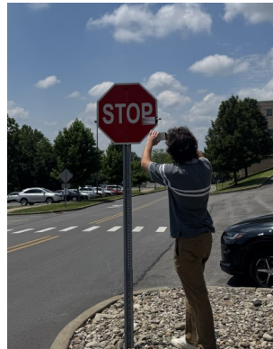
This photo showing panel use was taken during the day for clarity, but an actual inspection will need to be done at night.
