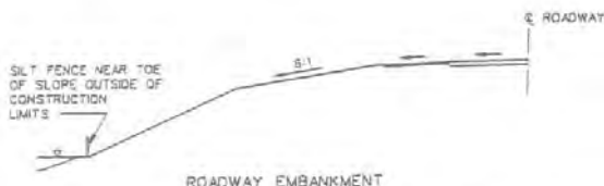
SILT FENCE TO PROTECT ADJACENT CRITICAL AREAS
