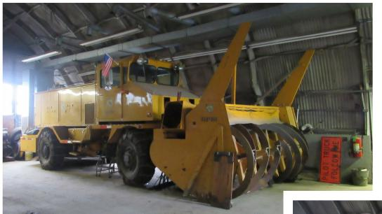
All mobilized snow fighting equipment should be started up monthly and exercised to insure it is in proper working condition
