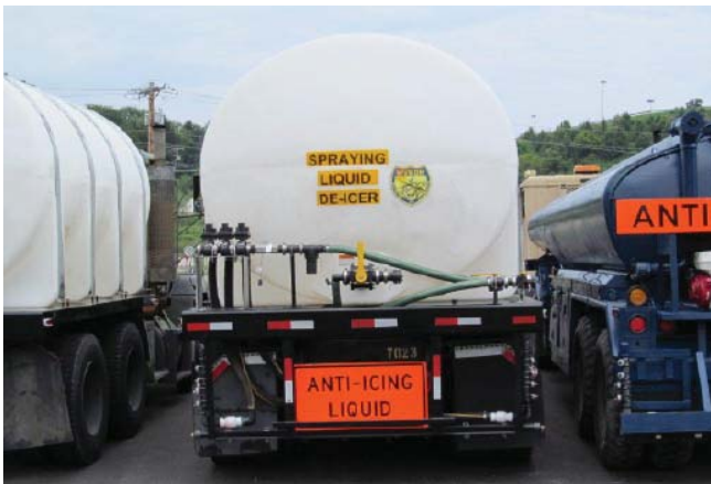
This photo taken by WVDOH D-4 staff shows three of their tanker trucks that are used for applying liquid anti-icers and de-icers.
