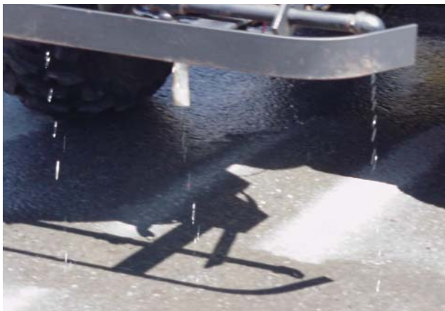
This photo taken by WV LTAP staff shows a spray bar that is attached to an ATV, used for treating walkways.
