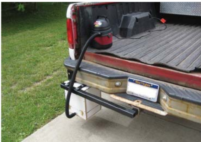
The mobile dust collector was used to determine the amount of dust released from the roadway when driven over.
