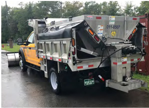
The WVDOH brought one of their new Ford F-550 Crew Cab 1 Ton dump trucks, with stainless dump body, stainless Henderson spreader insert, and Henderson plow. The specifications on these crew cab dump trucks will allow WVDOH work crews to travel to and from worksites more efficiently.
