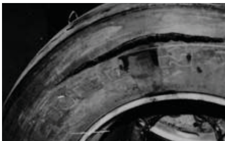
Zipper rupture on tire side wall.
