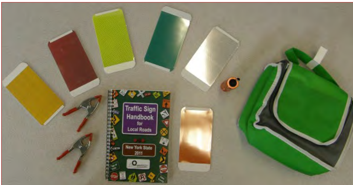
Completed Retroreflectivity Testing Kit
