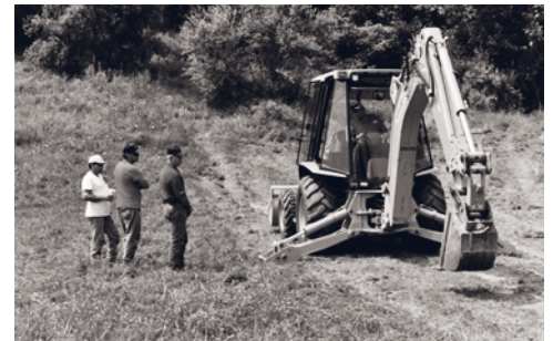
Donnie Morgan, from the City of Fairmont, practices using the stabilizers on a slope.
