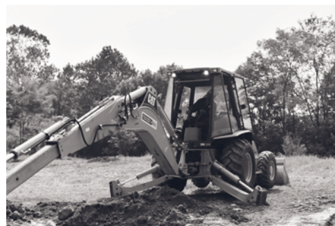
Roy Johnson, City of Morgantown, practices piling the dirt evenly along his trench.
